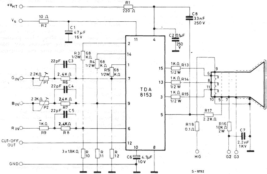
Fig. 9 - Application circuit for 30 AX CRT
