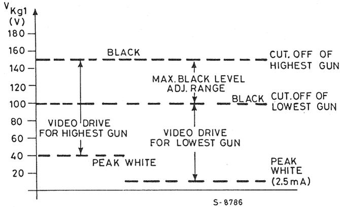
This minimum voltage is the sum of  $V_{g1}$ , of  $V_{gk}$  referred to the lower gun, of the voltage required to recover the difference of the cut-off values and of the higher saturation voltage of the amplifier.
